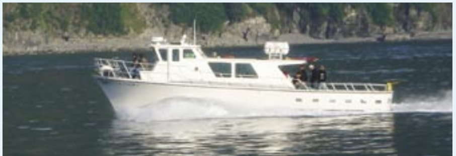
Seward Heavy Industrial Power installed a pair of Volvo Penta D9s in Aurora Charters' Delta 50 Emerald Fjord . The project set a new standard for Delta 50 repowers.
