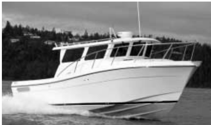
The new Ocean Sport Roamer sea-trialed at 44+ mph with twin KAD 44s.
